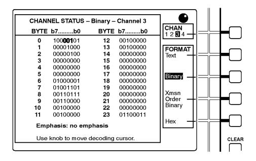
Figure 29: The Channel Status view, binary mode
